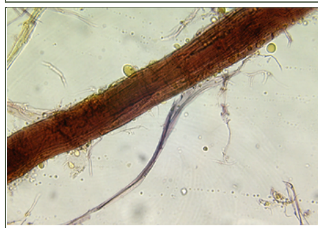
1.1: Ramie fibre stained with Herzberg observed in polarized light in magnification 300x.
