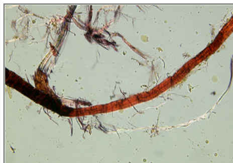
1.1: Ramie fibre stained with Herzberg observed in polarized light in magnification 300x.
